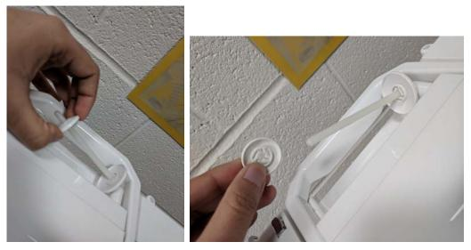
And then insert the top thread on the holder and add the top cap back. (This will lock the top thread in place.)
